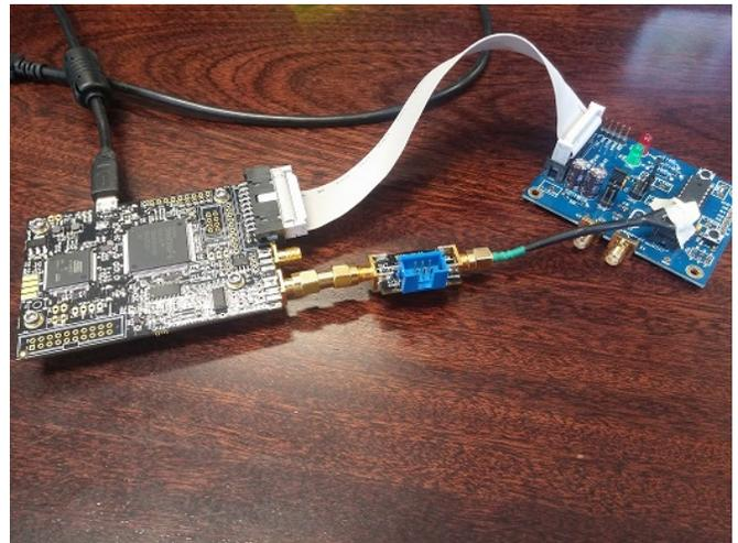
Fig. 1: The hardware setup: On the left, the ChipWhisperer connected to the PCB containing the Atmega328p processor; A low noise amplifier is connected to an EM probe placed on the processor.
